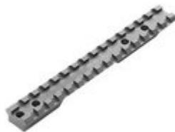
Heavy steel base with 20 M.O.A. forward angle increases maximum scope elevation for long range shooting. Machined after hardening to maintain dimensions. Integral recoil lug withstands the hardest kicking calibers. Uses MIL-STD 1913 Picatinny slot pattern for maximum sight mounting possibilities. Remington Zero Cant does not have 20 M.O.A. forward angle. For use where extra elevation is not required. Fits 700 short action only.
