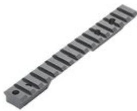
Heavy steel base with 20 M.O.A. forward angle increases maximum scope elevation for long range shooting. Machined after hardening to maintain dimensions. Integral recoil lug withstands the hardest kicking calibers. Uses MIL-STD 1913 Picatinny slot pattern for maximum sight mounting possibilities. Remington Zero Cant does not have 20 M.O.A. forward angle. For use where extra elevation is not required. Fits 700 short action only.
