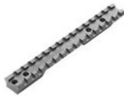
Heavy steel base with 20 M.O.A. forward angle increases maximum scope elevation for long range shooting. Machined after hardening to maintain dimensions. Integral recoil lug withstands the hardest kicking calibers. Uses MIL-STD 1913 Picatinny slot pattern for maximum sight mounting possibilities. Remington Zero Cant does not have 20 M.O.A. forward angle. For use where extra elevation is not required. Fits 700 short action only.
