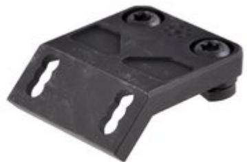
mounting surfaces of Picatinny handguards, the Offset Scout Mount places the light at a 45 degree angle and tucks it in closer to the rail system. Oriented upwards, the light is located at approximately the 1:30 or 10:30 clock positions. Oriented downwards, the light is located at approximately the 4:30 or 6:30 clock positions. Length: 1.30" / Weight: 0.7 oz Hardware: One 10-32x1.25" Torx cap head screw, two 8-32x5/16" Torx flat head screws.
